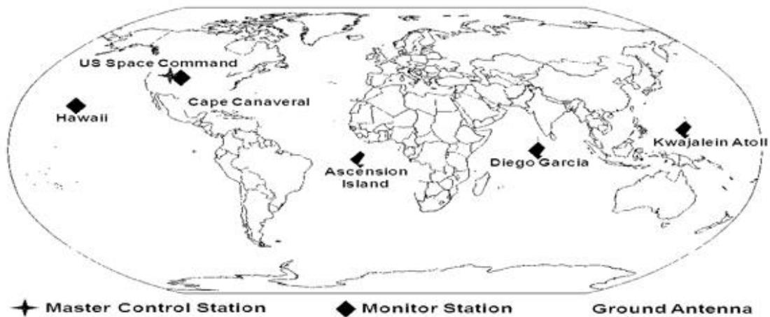
Figure: The Control Segment of the Global Position System
