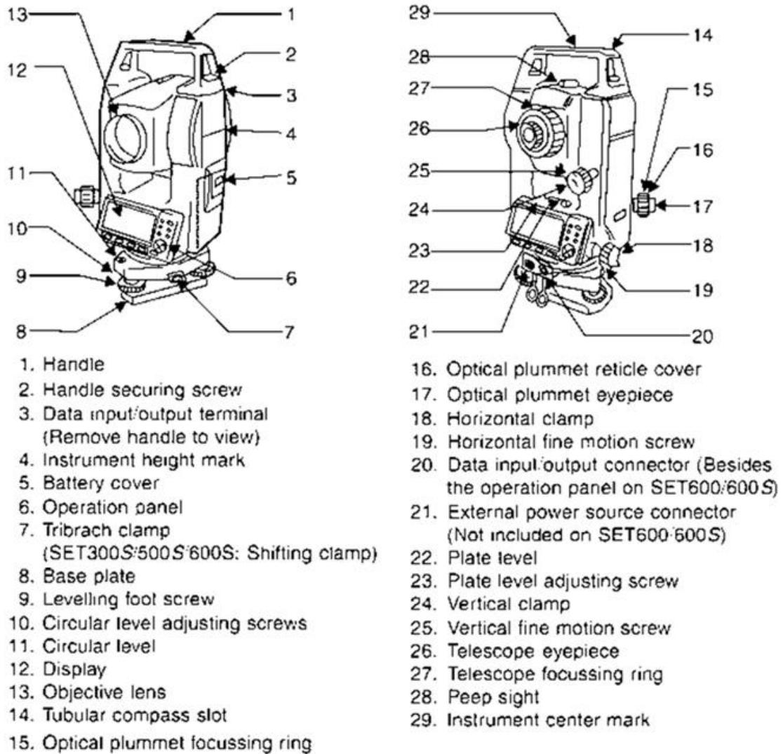
Figure: Basic Components of a Total Station
